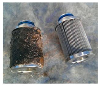
Common indicators that a microbial issue is occurring typically start with slowed fuel flow caused by filter plugging.
